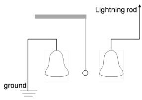
One of the two metal bells is electrically connected to the earth (ground) and the other is connected to a lightning rod. Between the two bells a metallic ball is suspended by an insulating thread.
